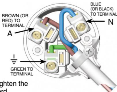
Note: Fit Adapter Piece (located between phase and neutral terminals) to cord clamp when using 2 core (0.75mm) flexible cord.
